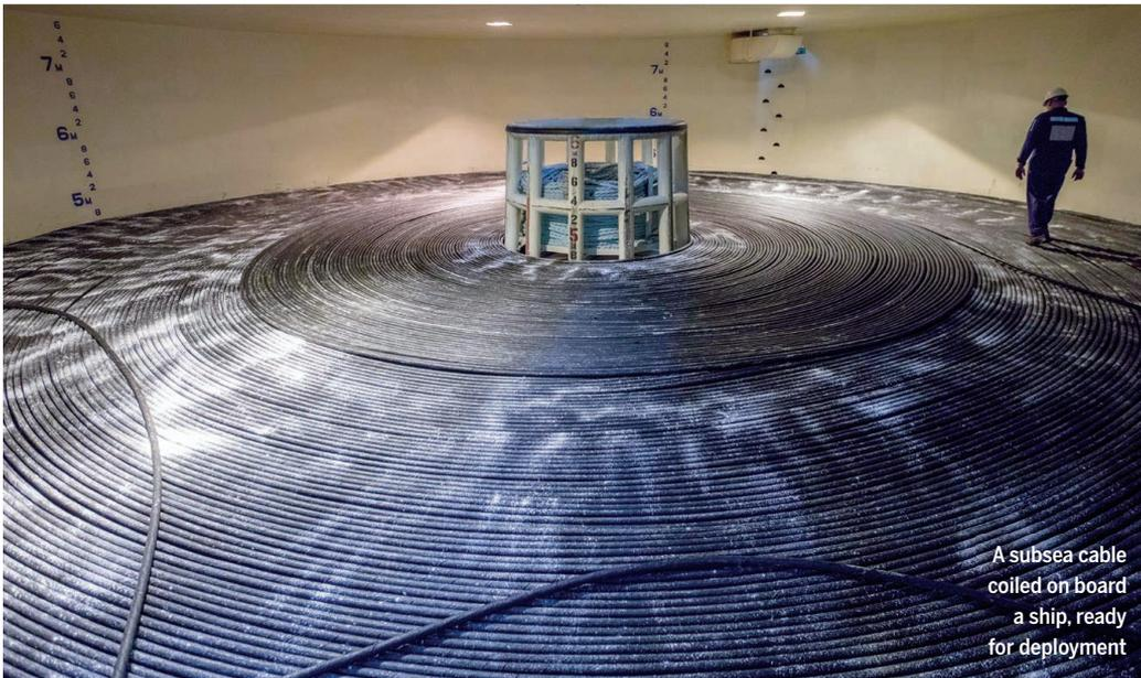
A subsea cable coiled on board a ship, ready for deployment
